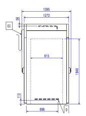
Drain Electrical inlet (power) RO Refrigerant Outlet
